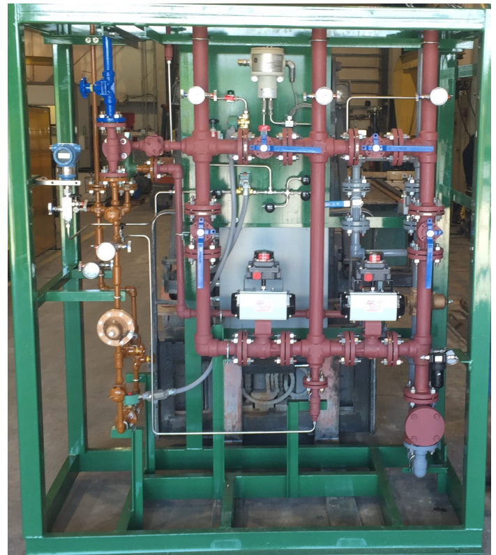
Generator Gas Monitoring and Control Skid (GMCP)
